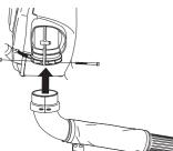
Also pay attention to the stops located on the pipe bend and the fan's outlet pipe. Ensure that the stop on the pipe bend comes in front of the stop on the outlet pipe.
